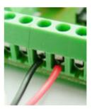
Stripped wires in a screw terminal.
