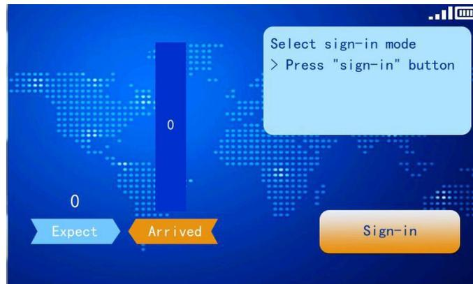
Press the sign-in button on the screen or press the switch microphone button to sign-in. After sign-in, the indicator light is always on, and the display is as follows:
