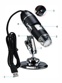
1. (The USB interface) 2. (LED lights) 3. (Ph oto button) 4. (Adj u st light brightness) 5. (U-shaped adjusting supp ort) 6. (Focusing roller) 7. (Height and Angle adjusting knob)
